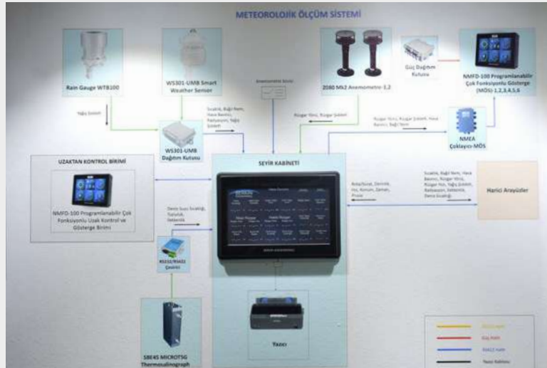
Meteorological Measurement System controls the meteorological sensors on the ship and facilitates communication between these sensors.
