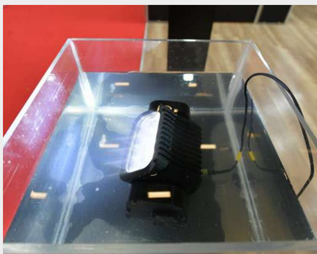
SHERPA projector stands out with its ability to rotate 360 degrees horizontally and vertically and operate underwater.
