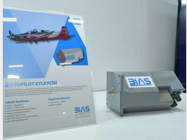
The autopilot actuator is indigenously developed to transmit commands from the pilot to the flight surfaces with appropriate speed and motion conditions.
