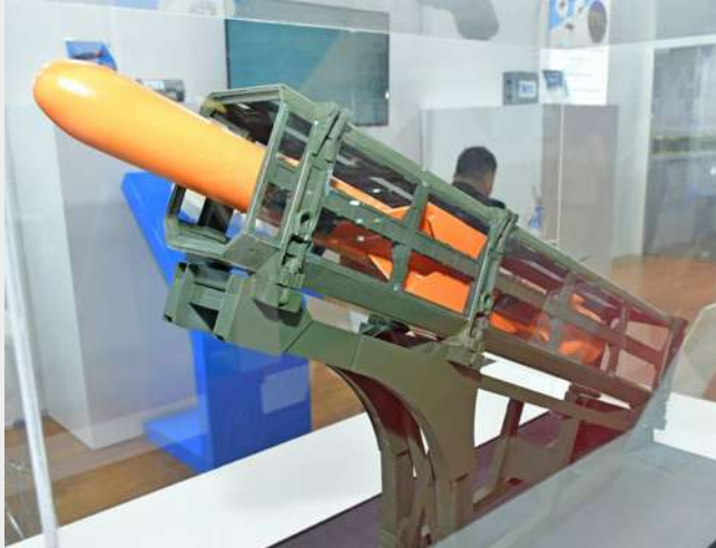
Canister system is used to launch guided munitions from land and naval platforms.
