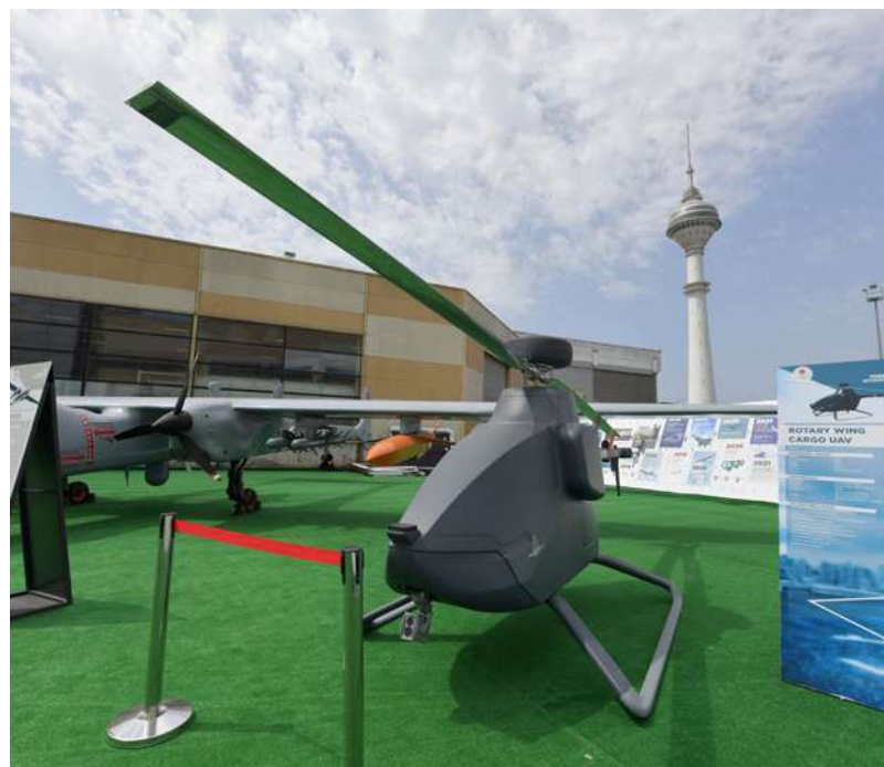
The rotary-wing UAV developed by Turkish Aerospace has a maximum take-off weight of 275 kg.
