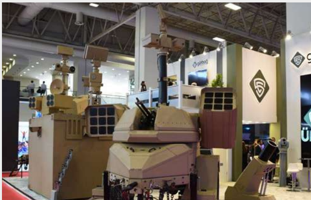
MM-GIDS can fire 1,500 rounds per minute with its triple-barrelled .50 calibre heavy machine gun.
